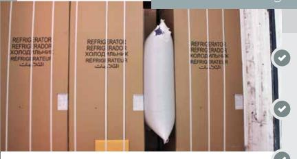
Container dunnage air bags, also known as "container air bags," are equipment primarily used in commercial shipping and the transportation of goods in containers. They stabilise cargo and protect goods from damage during transit.
